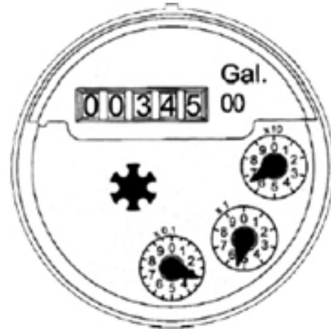
The 1700 Series counter consists of a row of numbers (roller counter) and one or more circular dials with rotating pointers. There is also a star shaped wheel that rotates whenever flow is present (trickle indicator).
