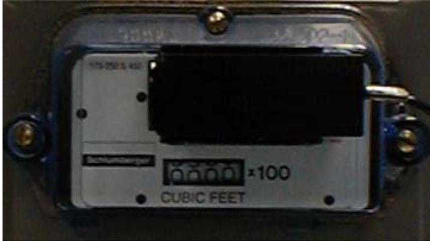
The DMP has a drive dog that engages one of the two test dials on the meter index. There are two test dials: one is ½ Cuft per revolution the other is 2 Cuft/revolution. The most common combination is to mount a 2 Pulse per revolution pulser onto the 2 Cuft test dial – this will produce 1 Pulse = 1 cuft.
