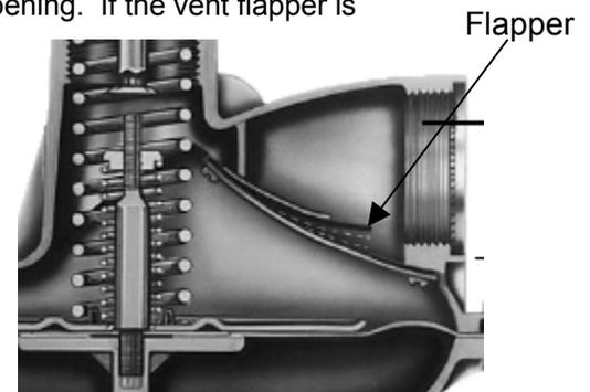
The Sensus/Invensys/Equimeter/Rockwell 243 series uses a round 2 way vent valve, the flapper disc is held in place with a set of light springs and rides on a stainless steel shaft. The two way design permits fast response to rapid changing loads.
