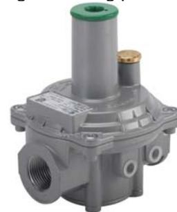
The line pressure regulator above does not have an OPD (over-pressure protection device) built into it. For CSA compliant systems, this regulator should only be used on inlet pressures of 2 PSIG or less and outlet pressures of 14" w.c. or less.
