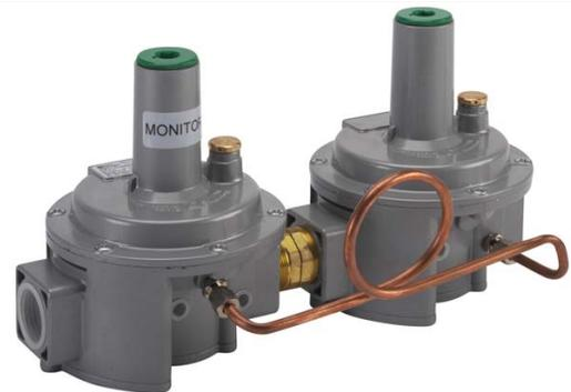
The line pressure regulator above employs an upstream wide open monitor. It senses the pressure being delivered by the downstream regulator. Should the downstream regulator fail open, the upstream monitor takes over and maintains pressure close to set point. This type of regulator is CSA certified for installation on systems up to 5 PSIG inlet and can be installed without a vent line if local authorities permit.
